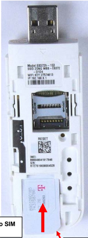
3- Approach modem with Micro SIM card . The chamfered corner is at bottom right.
