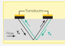
$T_F$ : time in flow direction  $T_R$  time in reverse flow direction
