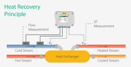
Heat exchangers transfer heat (energy) from a higher temperature medium (hot stream) to a colder one (heated stream). S461 measures the flow rate and the temperature difference between cold stream and heated stream. Based on these measurements the recovered energy will be calculated.
