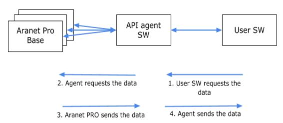
To limit the load of Aranet Pro Base stations, *aranet-agent* stores the gathered data in cache. The latest reading data from particular sensor are updated when new request from User SW arrives and data in cache are more than 60 seconds old.
