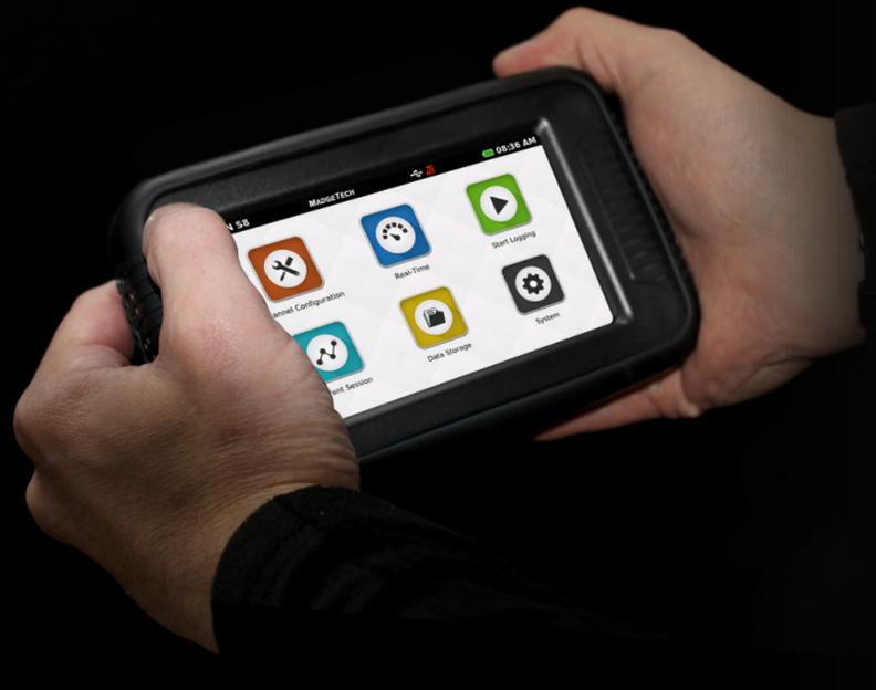
The MadgeTech Titan S8 is a portable, multi-use industrial data logger with eight probe channels and a user-friendly touchscreen interface. This versatile logger supports thermocouple, RTD or thermistor probes to measure current, voltage, temperature and pulse in real time. This adaptability and power make Titan S8 the perfect companion for any industrial engineer, quality assurance professional, compliance officer or automotive technician.
