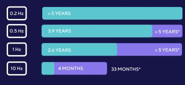
Results measured at room temperature under controlled circumstances. \*Battery life with auto-sleep feature enabled for tag being static 90% of the time, and static blink rate of 0.1 Hz
