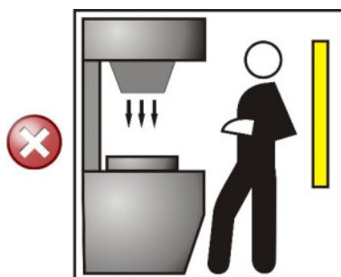
Figure 8: Wrong light curtain positioning
