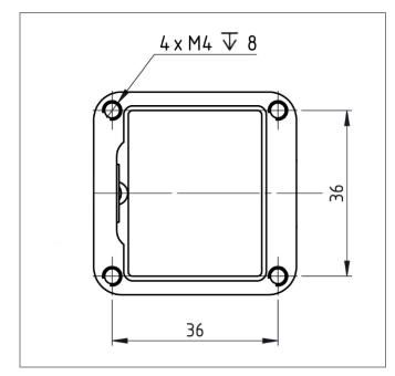
Dimensions of drill holes for mounting
