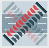
Transit-time principle for clamp-on flow measurement
